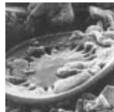
Microscopic morphology of diatomaceous earth - a key ingredient in most SeitzSchenk filter sheets
